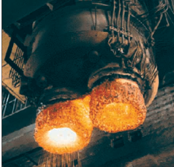
A vacuum degasser, showing the two snorkels at the bottom
