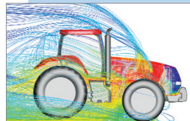
Airflow pathlines emitted from the hood grille of the virtual model
