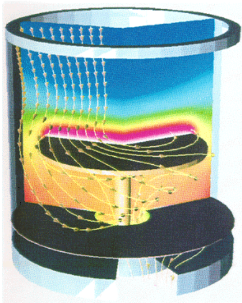
Figure 1. The 3-D model of initial MOCVD reactor conditions shows the sharp flow transition required for uniform film growth
