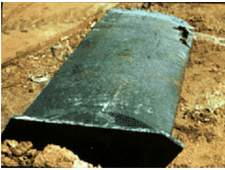
Fig 3. A real C 100 blade after four years' wear
