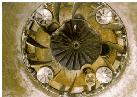
Radial and circumferentially staged coal flame stabilizer with RJM coal splitter.
