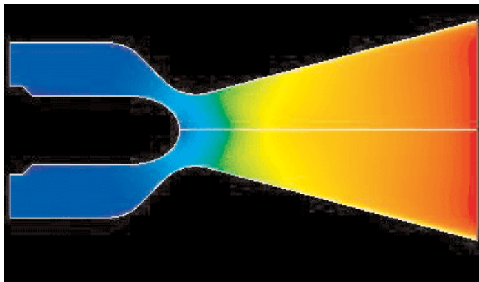
Figure 1: Mach contours for boost position, with the pintle fully open
