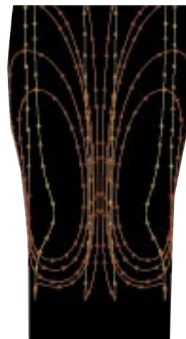
Bubble tracks show that the 1 mm bubbles (yellow) move steadily upwards while the 60 micron bubbles (red) are dragged downwards near the side of the glass.
