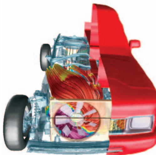
The flow generated by the front fan is shown in this cutaway view
