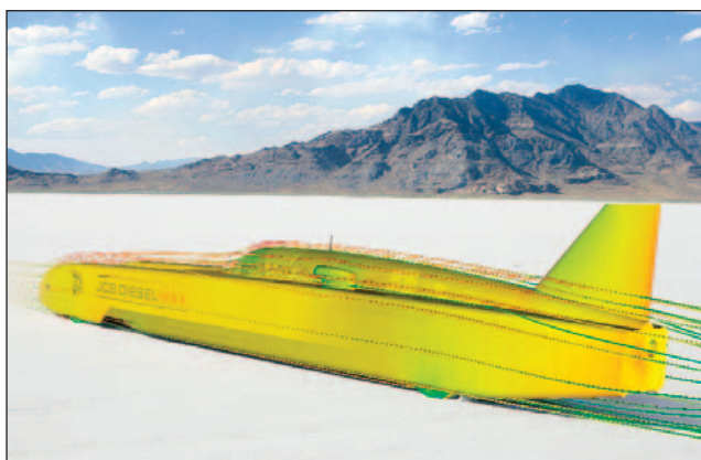
JCB DIESELMAX FLUENT model on the Bonneville Salt Flats with surface contours of static pressure and airflow pathlines colored by local flow velocity Courtesy of MIRA Ltd and JCB
