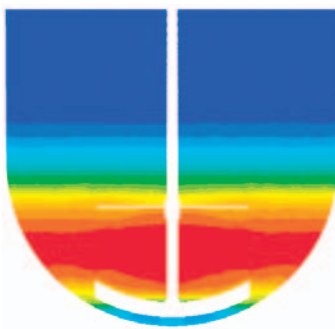
Volume fraction of water with the cyclotol/water interface at 20% of the liquid height
