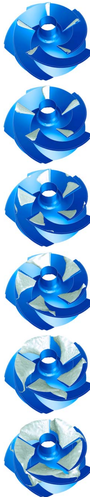
Iso-surfaces of water vapor for a pump operating with developing cavitation
