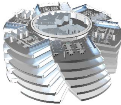
A CAD model of several floors in the Swiss Re building (left) and a CFD simulation showing airflow on one floor with windows open on the windward and leeward sides (right)
