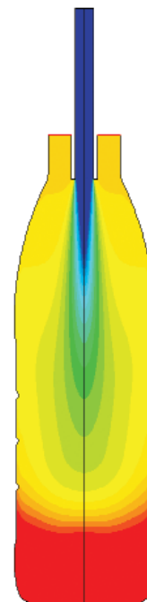
When flushing a bottle with hydrogen peroxide, it is essential that the air (red) be removed completely, as fast as possible
