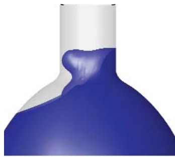
Simulation of bottle transport and sloshing for optimum machine configuration
