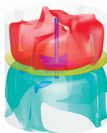
Iso-surfaces of tracer mass fraction show the polarized species distribution in the vessel, even after the liquids are well mixed
