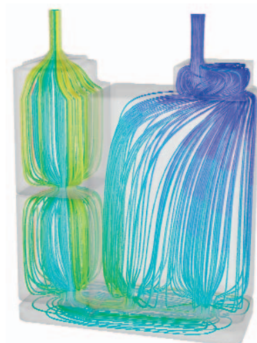
Pathlines show a dead zone in the upper left corner in the first carbon-filled chamber; the presence of dead zones points to underutilization of carbon
