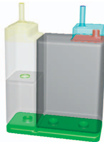
The geometry of the carbon canister, showing the inflow port (blue), 3 chambers packed with carbon pellets (gray) and vent port (yellow)
