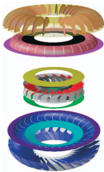
An exploded view of the torque converter showing the pump (top), stator (middle), and turbine (bottom)
