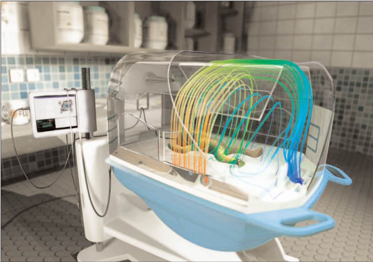
Pathlines, colored by temperature, illustrated the circulation inside the left side of the incubator Postprocessing courtesy of Michał Nowak
