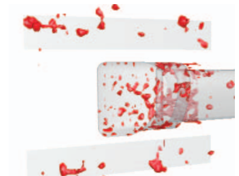
The water distribution for the modified scoop design shows that less water is directed into the air box
