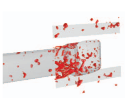
The water distribution for the modified scoop design shows that less water is directed into the air box
