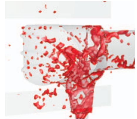
Iso-surfaces of volume fraction show the water distribution for the original scoop design
