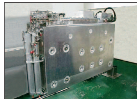
Extra long superconductors are used for magnet coils for maglev trains; the coils are cooled in units such as these
