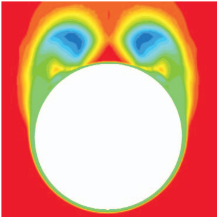
Contours of the normalized invariant of the deformation tensor in a cross-flow plane toward the rear of the spheroid; the RSTM-2 model was used with an incidence angle of 20°
