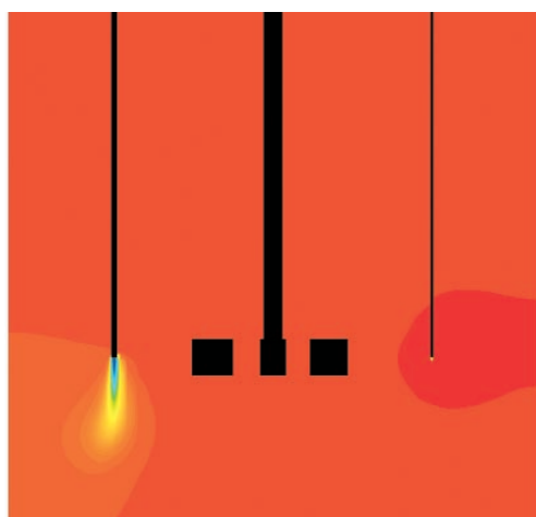
Contours of concentration of the secondary product S in the stirred tank reactor
