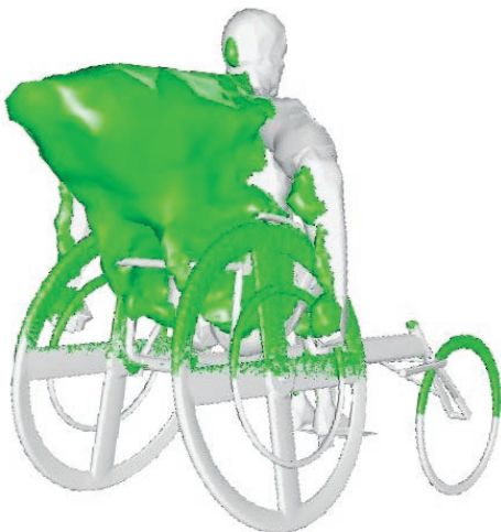
Recirculation zone behind the athlete after optimization of the wheelchair; the athlete is in an un-optimized position
