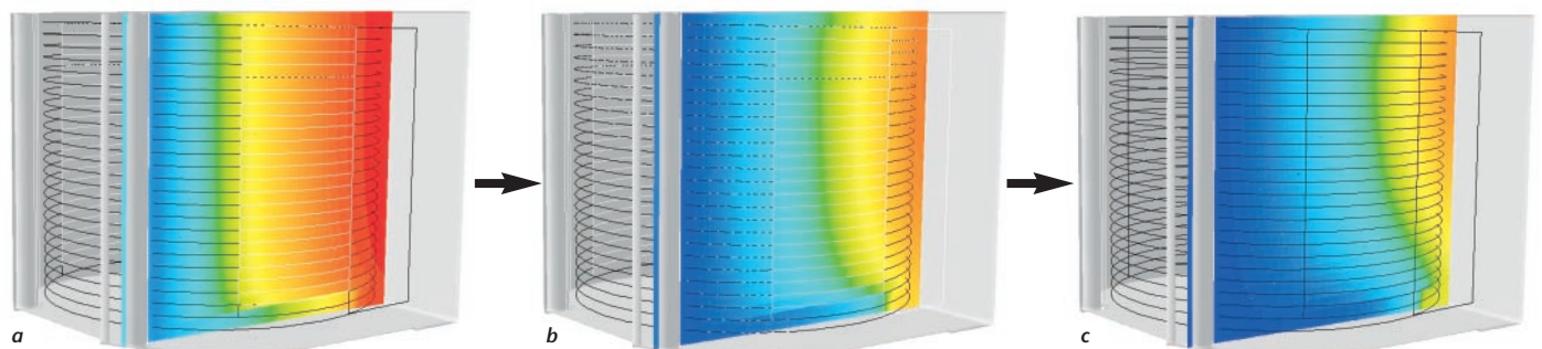
Mass fraction of the residual gas using plenum injector purging after a) 1.5 minutes, b) 5 minutes, and c) 22 minutes
