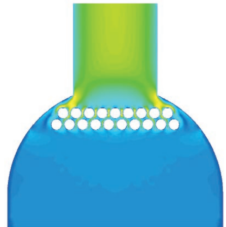
The rod grid (above) provides a fairly uniform distribution of velocity at the bundle entrance (below)
