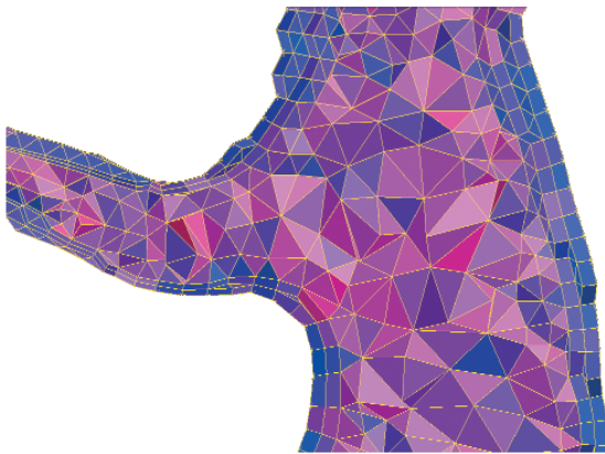
Generation of hybrid meshes of quadratic elements with adaptive boundary layer thickness for complex vascular tracts
