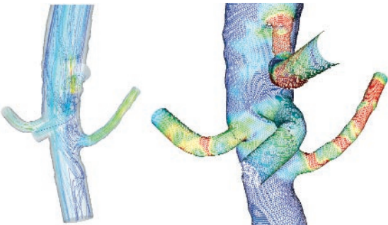
Time-dependent streamlines and wall shear stress distribution in a realistic model of an abdominal aorta
