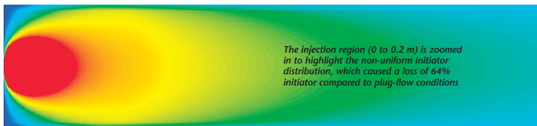
The mean mass fractions for initiator (top, 0 to 1.15 \times 10^{-3} ), monomer (middle, 0.95 to 1), and temperature (bottom, 250 to 307°C) inside a tubular reactor ( d = 3.8 cm, L = 10 m)
