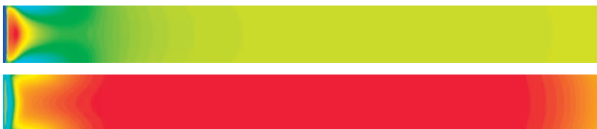
The effect of micromixing is shown through local temperature fluctuations in the reacting environment (top, 250 to 329°C) and higher polydispersity (molecular weight distribution) (bottom, 0 to 7.15)
