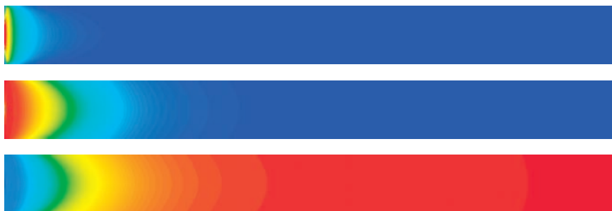
The mean mass fractions for initiator (top, 0 to 1.15 \times 10^{-3} ), monomer (middle, 0.95 to 1), and temperature (bottom, 250 to 307°C) inside a tubular reactor ( d = 3.8 cm, L = 10 m)
